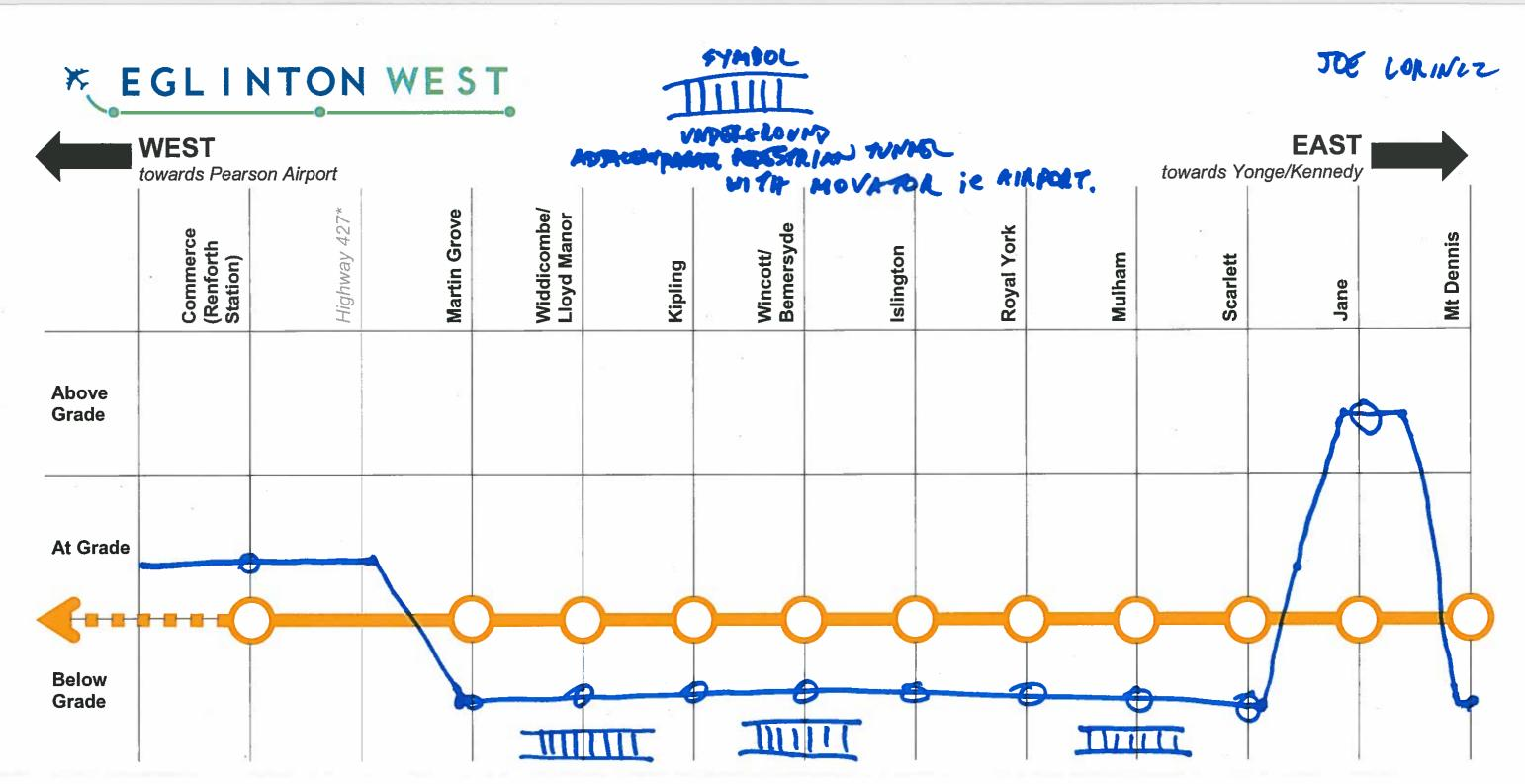
Use the above rows to draw what you believe is a feasible vertical alignment (whether above grade/elevated, at grade, or below grade) for each segment of the Eglinton West LRT. Each station/intersecting street is labelled above.
